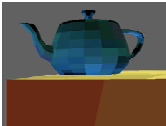
Figure 13: Detail of the reference scene obtained by traditional Monte Carlo radiosity after 1 step
