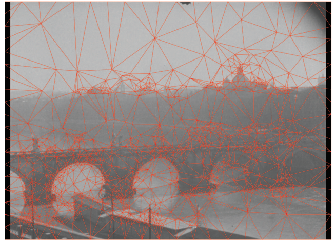
Figure 3: Motion adaptive warping mesh, superimposed on a reference frame from a panning sequence. By weighing the candidate vertices with the image gradient, nodal points are placed on strong image features.
