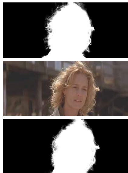
Figure 1. Harbor video sequence from [3]. Top: initial user-specified mask for frame #0. Middle: frame #30. Bottom: generated mask for frame #30 by forward-tracking the mask from frame #0 using the proposed algorithm.
