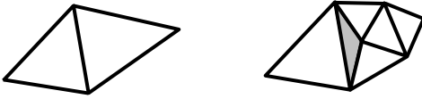
Figure 6: Left: two adjacent faces of the mesh. Right: one face is subdivided and the other is not, the crack between the faces is represented in grey.
