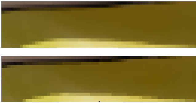
Figure 5: Quality comparison for 2 anti-aliasing presets: FLIPQUAD with 16 additional per-pixel samples (upper image) and FLIPTRI with 4 samples shared for 2x2 pixels block (lower image). The performance difference is not very high (just 2X) due to better ray coherence of the FLIPQUAD-based preset.
