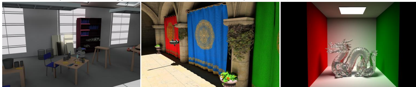
Figure 1. The presented screenshots were rendered at 1920x1200 resolution on a GTX 560 HW under 5 minutes using Irradiance Caching (IC) technique. We achieved from 5 to 15 times acceleration compare to our naive path tracing implementation.
