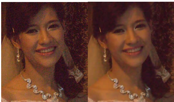
Fig. 11 Face high ISO digital image after proposed edge bilateral filtration ( N=6 , \sigma=900 )
