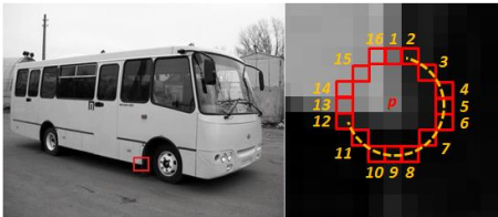
Figure 1: Definition of corners by means of the detector FAST with the radius of a considered circle of 3 pixels. Intensity of the pixels lying on a dashed line are less than central pixel p intensity by a set threshold t , 0 < t < 255 .
