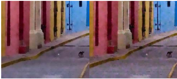
Fig. 9 Caracas noised image after bilateral filtration (left) and after proposed edge bilateral filtration (right)
