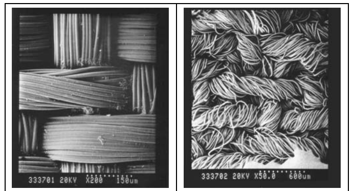
Fig.1. Woven textiles received via scanning electronic microscope Hitachi S800.
