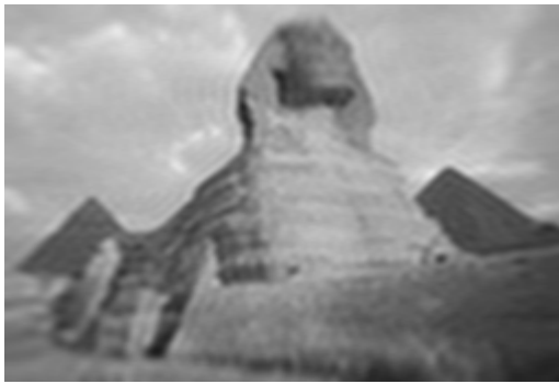
Figure 12: 2D decoded image by 80 Hermite functions at the first pass and 60 Hermite functions at the second pass
