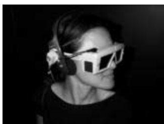
Figure 16: Shutter-Glass + Headphone + Tracker (CrystalEyes, Inc.)
