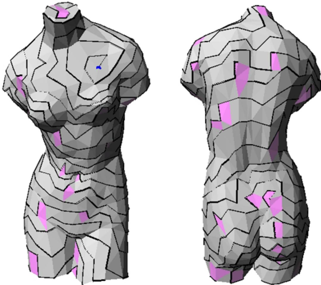
Fig.3. The above figures depict the order of vertex traversal generated by our algorithms (black solid lines). The blue dot is the initial vertex  $r_1$ . Notice that while the order of traversal does not necessarily form a path on the graph of the mesh, a large proportion (99.7% in this example) of adjacent vertices  $v_i v_{i+1}$  indeed form edges of underlying graph.
