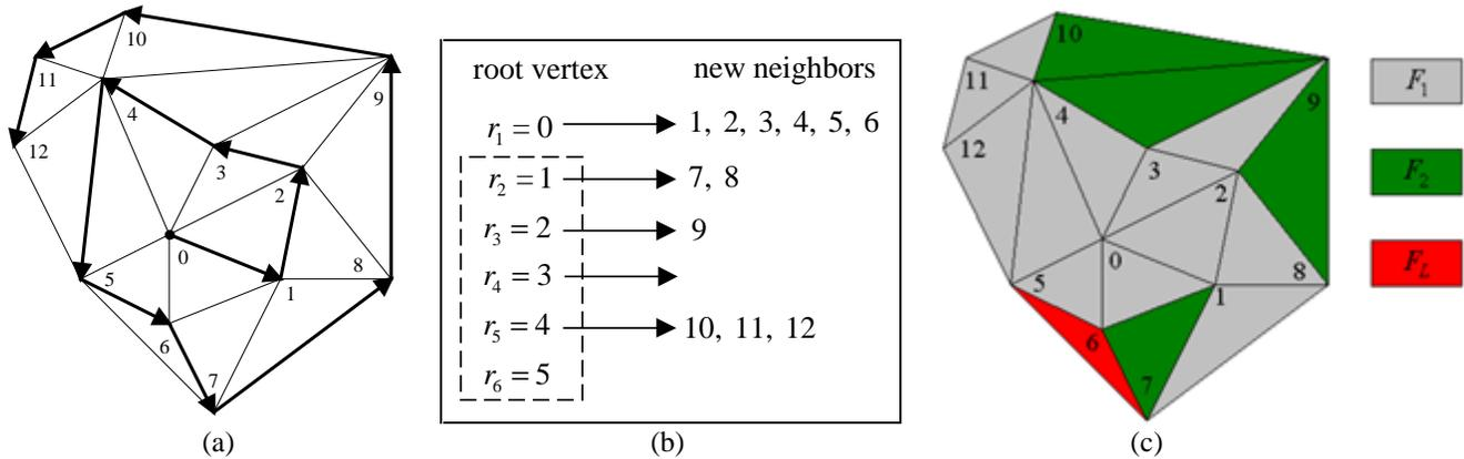
Fig.1 (a) Vertex traversing and reordering; (b) Trimmed Adjacency lists; (c) Connectivity encoding.
