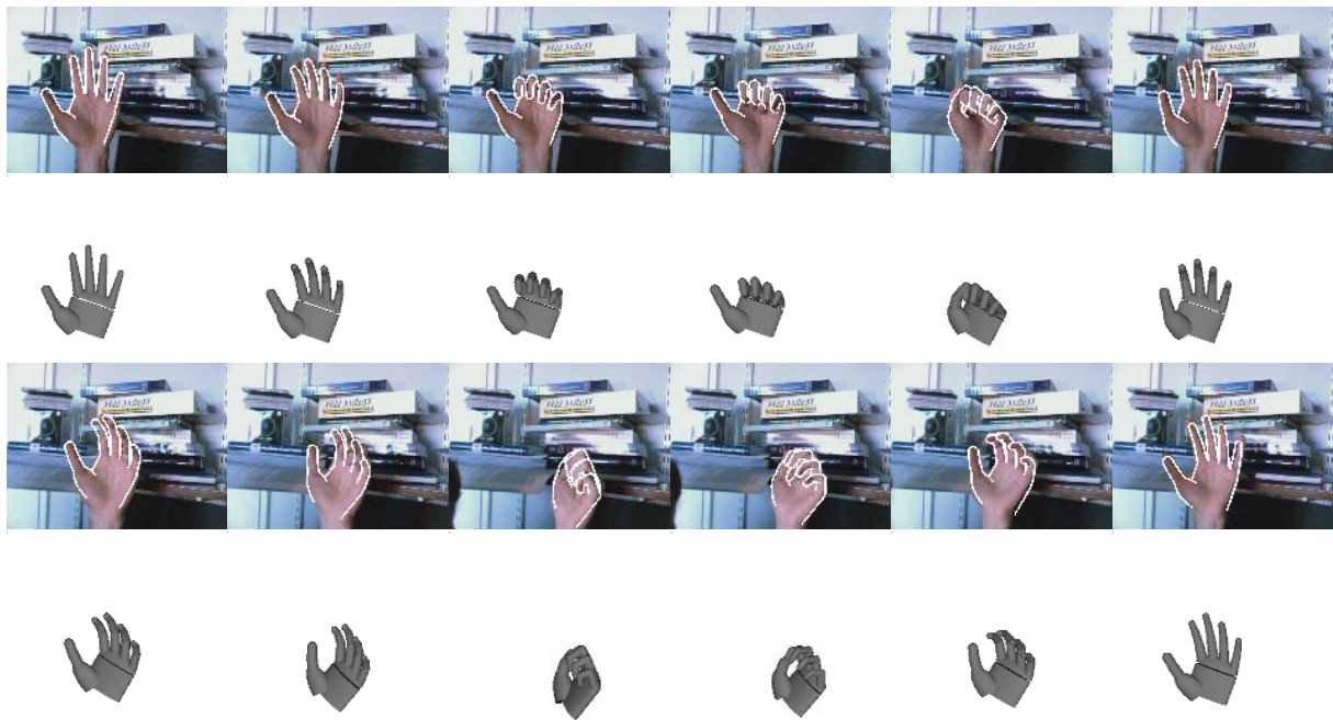
Figure 13: Tracking a hand opening and closing with rigid body motion in front of clutter. In this sequence 6 DOF for rigid body motion plus 2 DOF for finger flexion and extension are tracked successfully.
