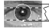
Figure 5: Detection of the eye opening height with row-by-row analysis of average iris luminance
