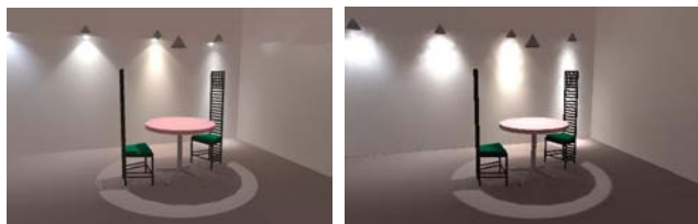
Figure 7: Illumination maps and shaded textures. Left – raytracing, right - OpenGL rendering (a lighting texture was applied to the floor)
