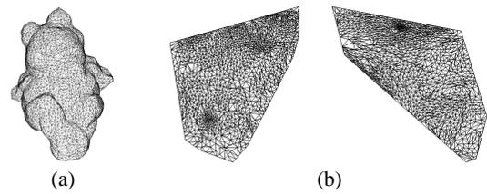
Figure 8: Mesh of Frog and its parametrisation.
