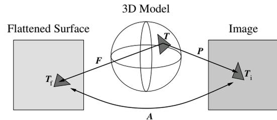
Figure 9: Relation between 3D model, optical image and flattened surface.  $T$  is a triangle,  $F$  flattening,  $P$  projective mapping,  $A$  affine mapping.
