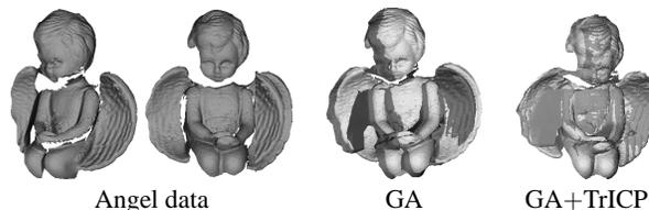
Figure 3: The Angel dataset, GA alignment and final alignment.
