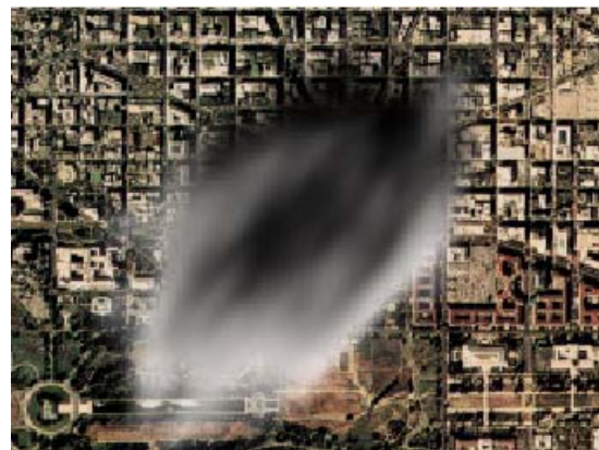
Figure 1: Taking into account only single scattering of light inside cloud leads to abnormal dark parts on the opposite side from the light source [4].
