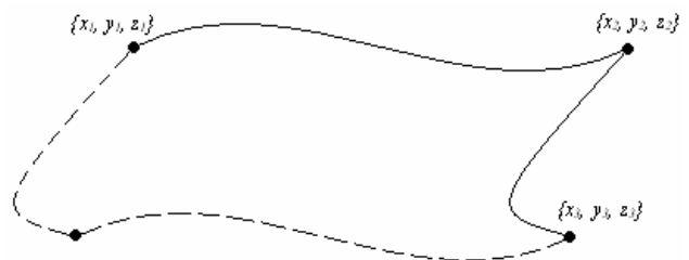
Figure 6: Missing edges construction – two adjacent edges.
