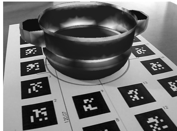
Figure 4. Real pot augmented with stress simulation.
