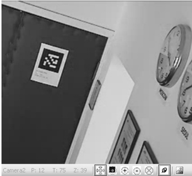
Figure 5: ARTag visual marker acting as a calibration object
