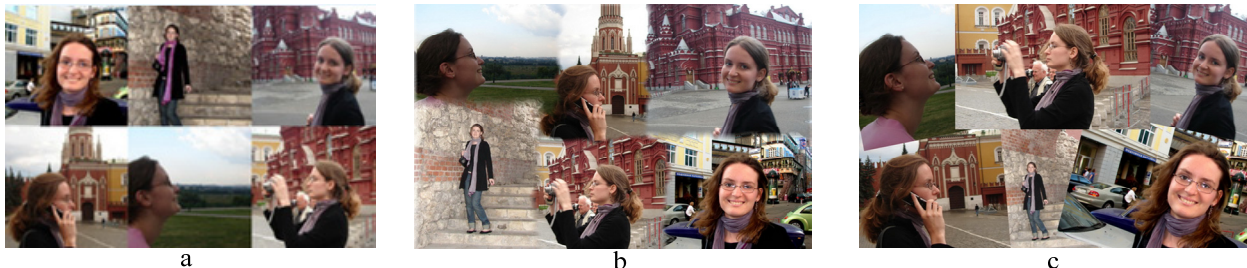
Figure 1 Collage comparison. Three ways to create a collage: (a) tiling collage, (b) collage with blending, (c) picture collage
