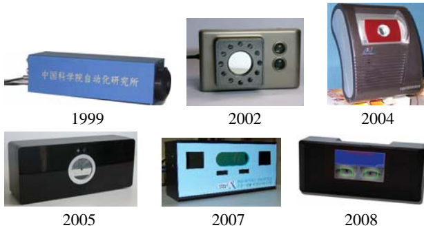
Figure 5: Close-range IR cameras developed by CASIA.
