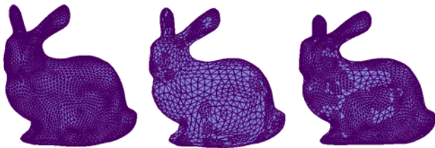
Figure 13: From left to right: respectively full subdivision, adaptive subdivision with an accuracy of 0.1, adaptive subdivision with an accuracy of 0.05.
