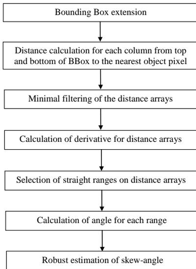
**Figure 3:** General scheme of skew-angle estimation.
