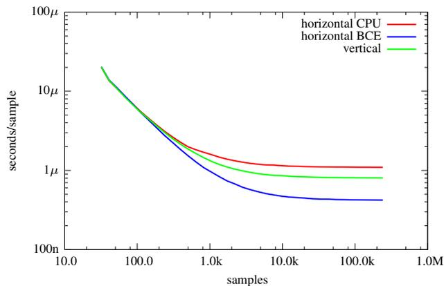
**Figure 6:** Comparison of three described approaches on the ASVP platform. The horizontal parallelization was implemented on the CPU as well as on the BCE unit. Using the BCE unit, horizontal parallelization is clearly the fastest method with up to 2.6× speedup.
