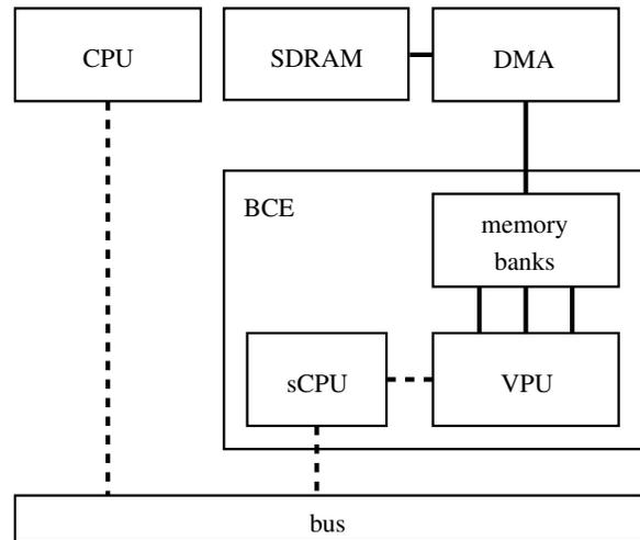
**Figure 1:** Organization of ASVP platform. Solid lines indicates data paths. In our case, function of BCE is controlled by host CPU (MicroBlaze). The sCPU means for simple CPU what is the PicoBlaze processor here. Moreover, the BCE element consists of four memory banks, each 1024 32-bit words long, and Vector Processing Unit (VPU) which performs actual operations. The BCE accesses RAM through DMA engine.
