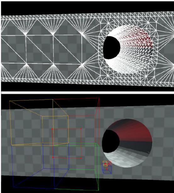
Рис. 1: Surface extracted from an implicitly-defined object using adaptive dual contouring. The lower image shows octree cells in the uniform and adaptive case.
