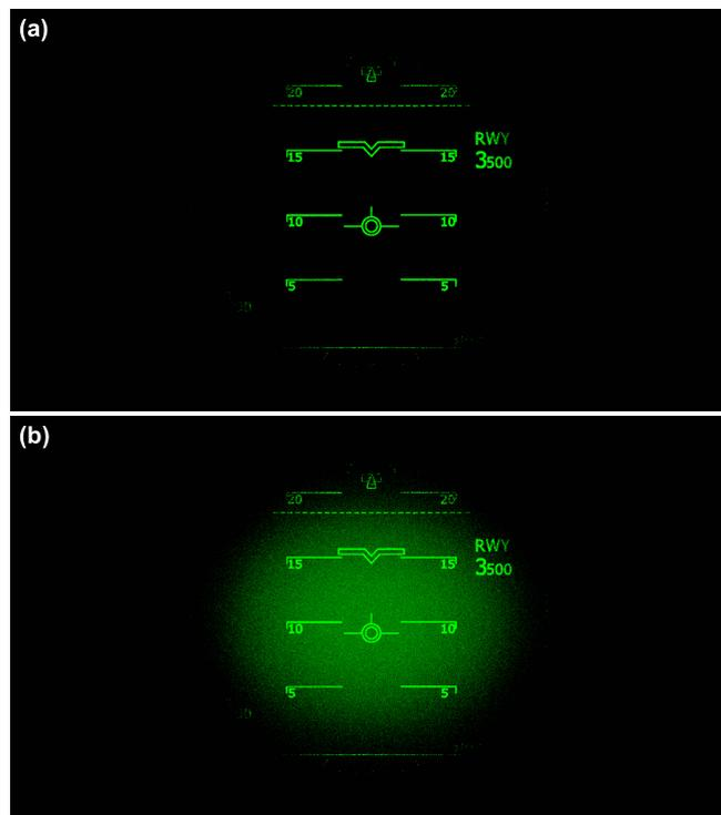
**Fig. 10.** The HUD image simulation result for case (a) LCD with absolute contrast and (b) LCD with real contrast.
