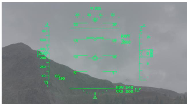
**Fig. 9.** Example of AR image synthesis for optimal selection of the LED brightness level.
