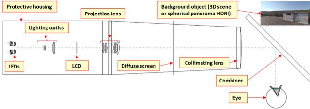
Fig. 2. Scheme with the intermediate diffuse screen.
