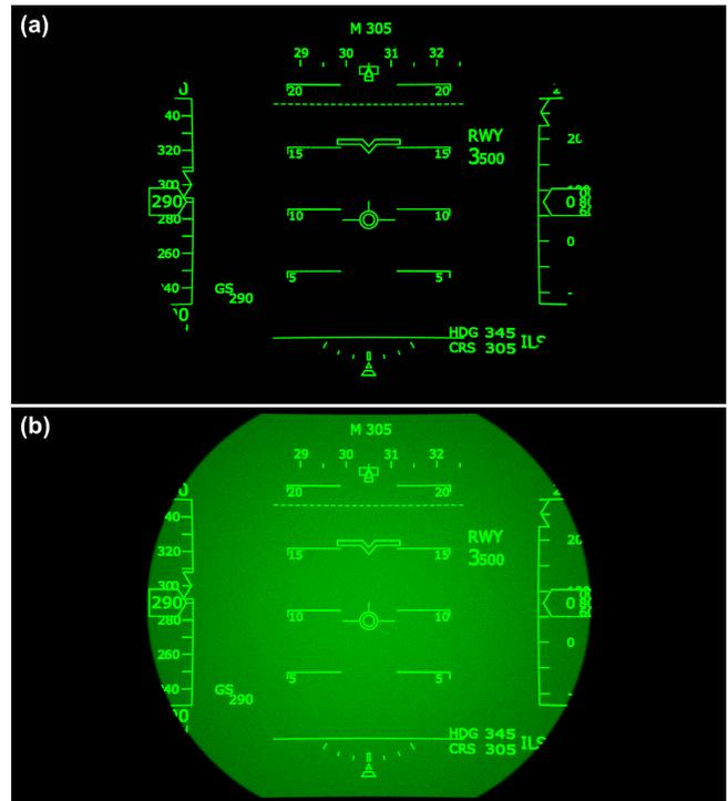
Fig. 6. The HUD image simulation result for case (a) LCD with absolute contrast and (b) LCD with real contrast.
