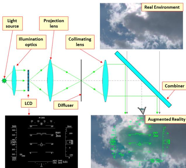
Fig. 1. Principal scheme of HUD with LCD source.
