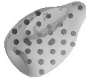
**Figure 8:** Sample surface (transparent) with a pseudo-atom grid inside.
