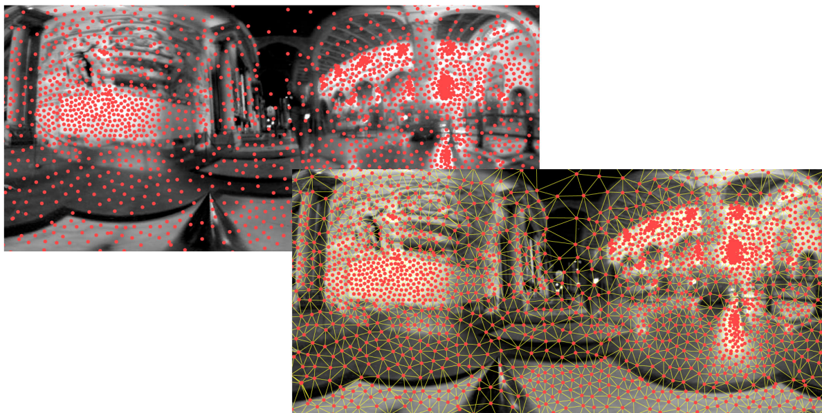
Figure 10: HDR map sampled with the Penrose-tiling-based sampling system (background image), then triangulated using our algorithm (foreground image). The total running time was 0.094 seconds on a P4 at 2.6 GHz. Running time is linearly proportional to the number of vertices. HDR image source: Paul Debevec.
