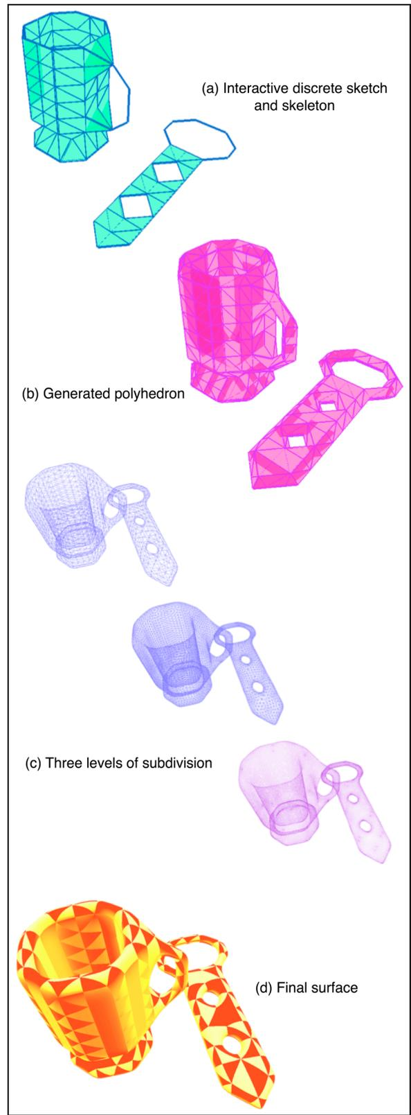
**Figure 18:** Mesh generation of a mug and a bottle-opener.
