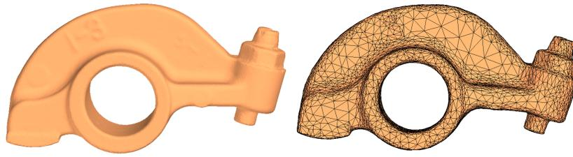
**Figure 8:** The rocker arm model simplified by our method: initial model, 40k vertices (left) - simplified model, 5k vertices,  $D_{max} = 0.00029$ ,  $D_{avg} = 0.0000345$  (right) - size of the uniform grid:  $41 \times 24 \times 78$ , size of the intermediate mesh: 20088 vertices
