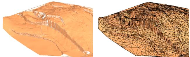
**Figure 9:** A geological surface simplified with our method: initial model, 112k vertices (left) - simplified model, 3k vertices - size of the uniform grid: 151x188x27, size of the intermediate mesh: 56136 vertices
