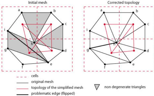
**Figure 7:** Heuristic for the well known topological problem (non-manifoldness): left, the original mesh - right, the corrected mesh (an edge has been flipped) which gives rise to a manifold simplified mesh
