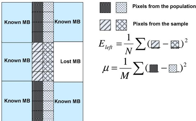
Figure 4: **Boundary Error Estimation Scheme for Left Boundary**
