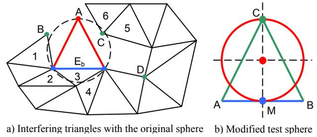
**Figure 3:** Interfering triangles with the original Delaunay sphere and modified test sphere
