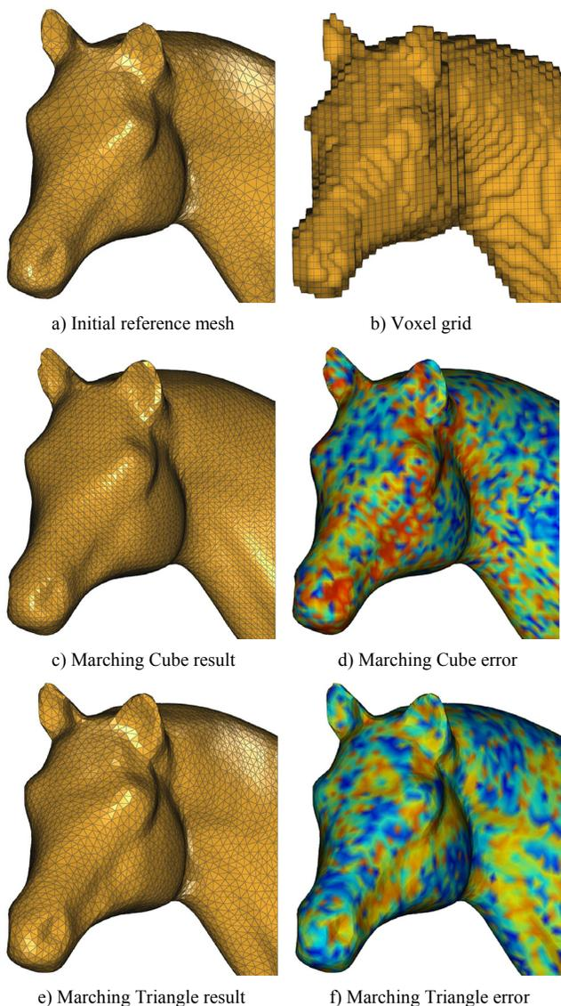
**Figure 10:** Triangulation results on the Horse model
