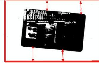
**Figure 4:** Distances from top and bottom of extended bounding box to the nearest foreground pixel.
