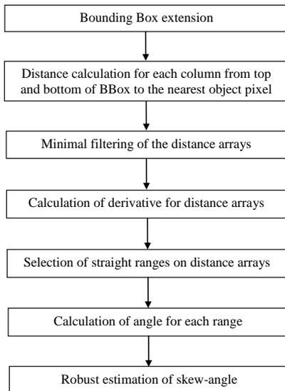
**Figure 3:** General scheme of skew-angle estimation.
