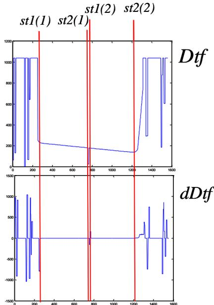
Figure 5: Distance and derivative of distance arrays.
