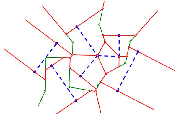
Fig. 2. The control graph of the Voronoi diagram of line segments (dotted line): line Voronoi edges (red) and control polygon edges (green)
