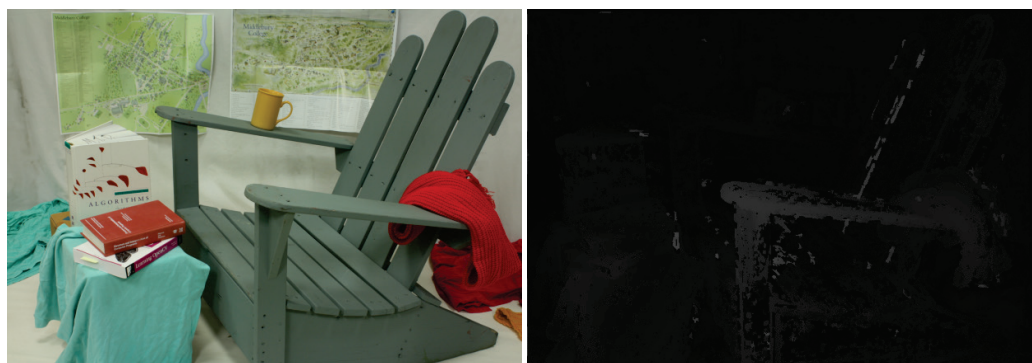
Figure 1: The testing image from one of the sensors of the stereo system on the top and the depth map calculated by the presented algorithm on the bottom
