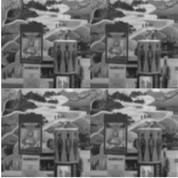
Figure 1: A stereo image sequence with known parameters of \mathbf{T} = (1.0, 1.65, -1.8)^T cm and \mathbf{W} = (0.029, -0.016, 0.0)^T : (a) and (b): left and right image of the second stereo pair, (c) and (d): left and right image of the first stereo pair
