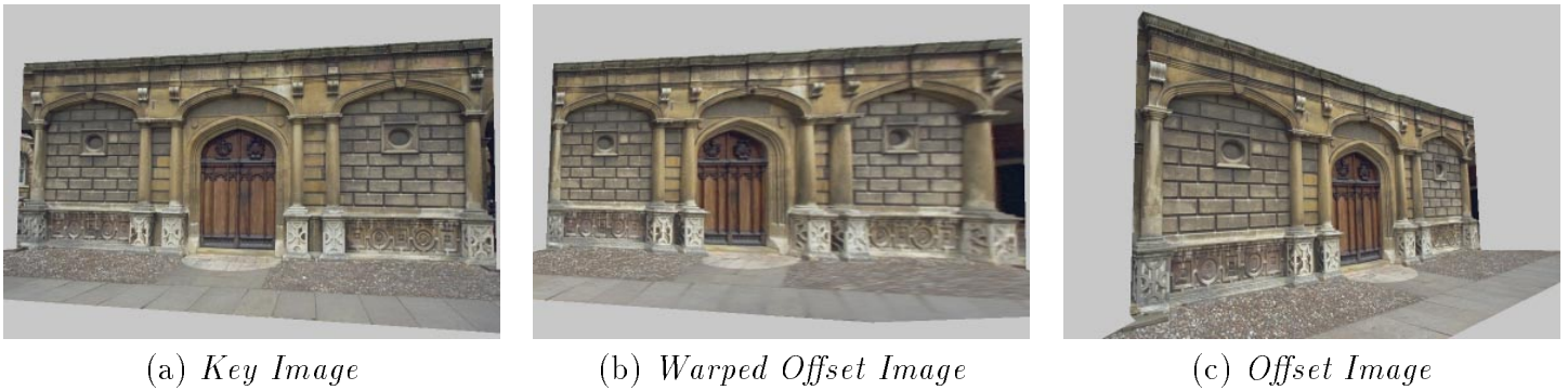
Figure 16: (a) and (c) are two pictures of the entrance to the Peterhouse college chapel in Cambridge, England. The Façade system was used to model the façade as a flat surface and to recover the relative camera positions. In (b), the warped offset image is produced by using the offset image to texture map the geometric model as viewed from the position of the key image. In our model-based stereo approach, correspondence is performed between the key and warped offset images instead of the key and offset images. This is advantageous because the key and warped offset images are typically very similar in appearance; any differences are due to the unmodeled geometric detail.
