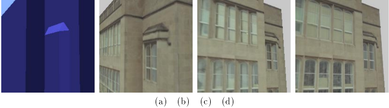
Figure 14: View-dependent texture mapping. (a) A detail view of the high school model. (b) A rendering of the model from the same position using view-dependent texture mapping. Note that although the model does not capture the slightly recessed windows, the windows appear properly recessed because the texture map is sampled primarily from a photograph which viewed the windows from approximately the same direction. (c) The same piece of the model viewed from a different angle, using the same texture map as in (b). Since the texture is not selected from an image that viewed the model from approximately the same angle, the recessed windows appear unnatural. (d) A more natural result obtained by using view-dependent texture mapping. Since the angle of view in (d) is different than in (b), a different composition of original images is used to texture-map the model.
