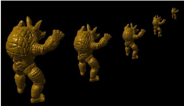
Figure 11: Levels of detail of the armadillo model shown with 1.0 mm maximum image deviation. Triangle counts are: 7,809, 3,905, 1,951, 975, 488
