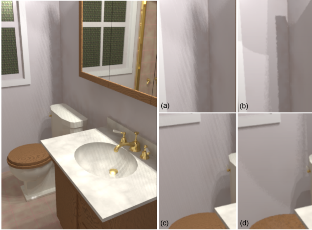
Figure 12: The image on the left is rendered using the baseline RADIANCE system by setting the quality to the highest level available. On the right, (a) and (c) are zoomed views of two regions from the left image. Notice the striping artifacts and missing penumbra boundaries. In (b) and (d), we show zoomed views of the same two regions from an image rendered in less time by our progressive renderer (for the complete image see the Conference Proceedings CD-ROM). The scene model was provided courtesy of Greg W. Larson.
