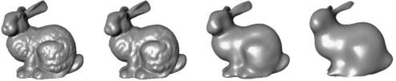
Figure 7: Four versions of the Stanford bunny. On the left the original data set. In the center left the same object after 200 iterations of the non-shrinking Laplace-filter. On the center right and far right the original data set after applying the multi-level umbrella filter with three or six levels respectively.
