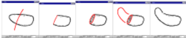
a) cutting stroke b) result c) rotated d) extruding stroke e) result
