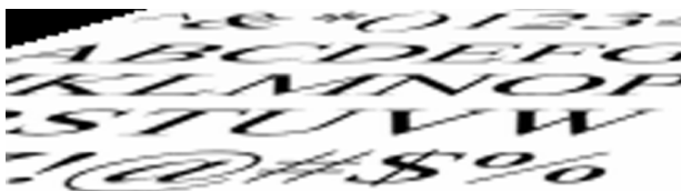
Figure 20: Texram paints text with stairstepping.
