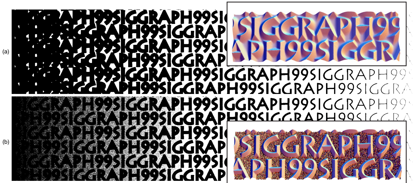
Fig. 4 Grayscale wedge produced (a) with a standard continuous dither matrix and (b) with a mixed dither matrix made of partially continuous, partially random threshold levels.
