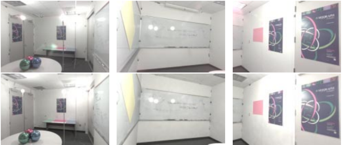
Figure 13: A comparison between real images (top) and synthetic renderings of our room with the recovered reflectance parameters (bottom). The simulated lighting is the same as in the original pictures, and the synthetic viewpoints have been matched to the recovered camera positions of the real images. The images show that good consistency was achieved.
