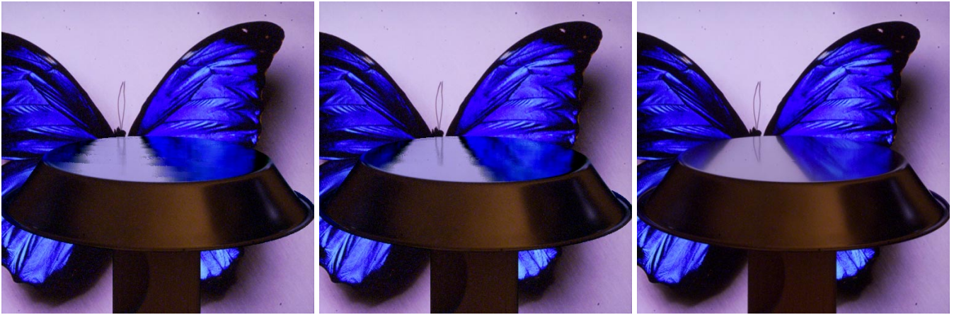
Figure 6 An object with glossy reflection, captured using an environment matte. From left to right: artifacts produced in composite image when the box filter approximation is used during acquisition, the improvement produced when a Gaussian approximation is used instead, and the actual photograph.
