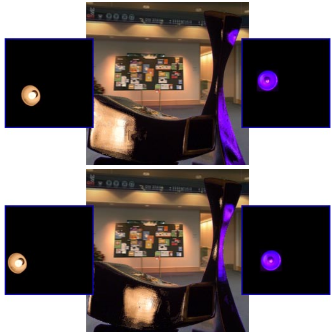
Figure 8 Interactively relighting an object, using photographs of lights as sidedrops. The left and right sidedrops (shown in insets) are generated by moving a picture of a light source around within the texture map.
