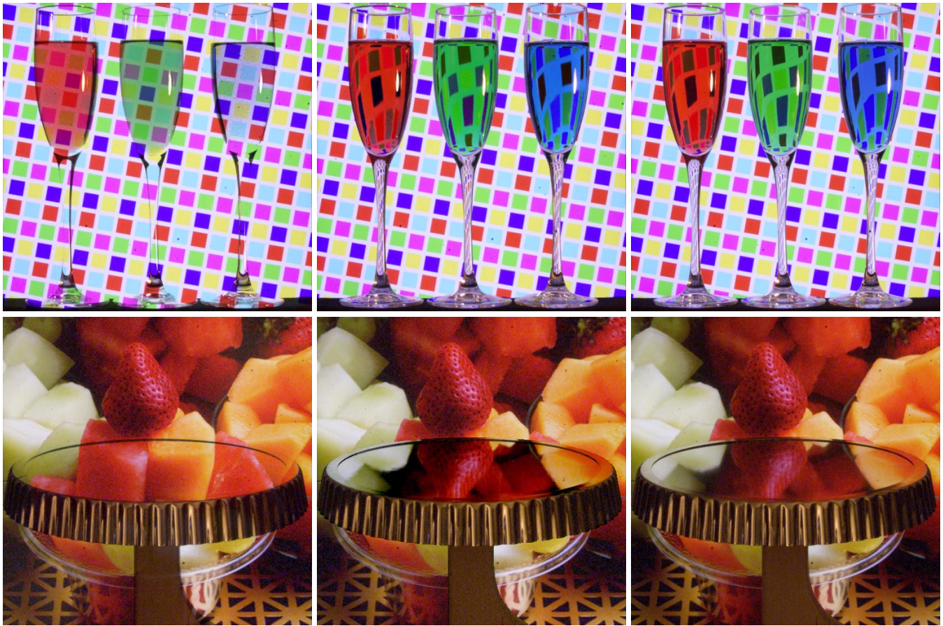
Figure 5 From left to right: an alpha matte composite, an environment matte composite, and a photograph of an object in front of a background image. The top row shows three glasses of water tinted red, green, and blue; the bottom row shows a pie tin tilted to reflect light off the backdrop.
